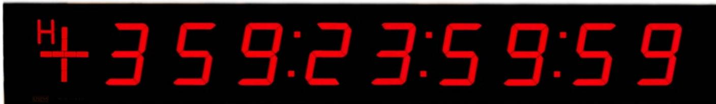
The TCR-495 provides a large, easy to read visual display of IRIG-B, IRIG-CS3, MILA/KSC, CCS, FDME/BUDX, and IRIG-CS5 time and countdown codes.
