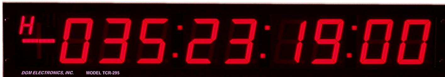
The TCR-295 provides a large, easy to read visual display of IRIG-B, IRIG-CS3, MILA/KSC, FDME/BUDX and IRIG-CS5 time and countdown codes.
