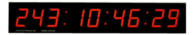
The TCR-290 has been designed to automatically select and display IRIG-B120, FDME/BUDX, KSC/MILA and IRIG-CS3 time codes. It also displays IRIG CS-5246, CS-5347, CS-5248 countdown formats. Two digital inputs (IRIG CS-5) are provided. One for RS-232 voltage level data and the other for RS-422 level data. A DIP switch on the rear panel is used to select between the analog or digital codes, selection of IRIG CS-5 inputs, and IRIG CS-5 display formats.
